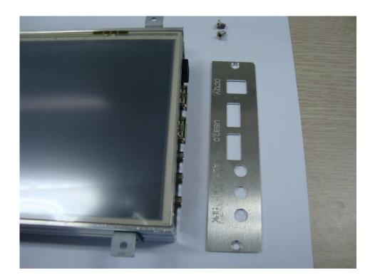
2. LCD Separation – LCD Connector Separation
