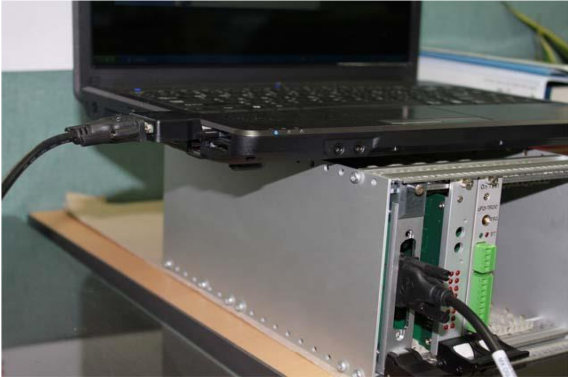
[Figure 1-2. eCard-LK02 & Compact PCI System Connection]
